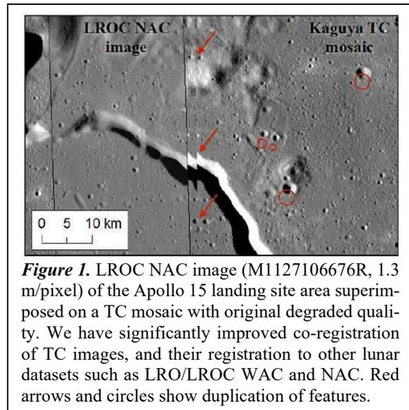
*Figure 1.* LROC NAC image (M1127106676R, 1.3 m/pixel) of the Apollo 15 landing site area superimposed on a TC mosaic with original degraded quality. We have significantly improved co-registration of TC images, and their registration to other lunar datasets such as LRO/LROC WAC and NAC. Red arrows and circles show duplication of features.
