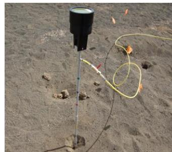
Figure 7. Pneumatic deployment of a corner cube reflector.
