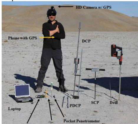
Figure 5. Geotechnical tools deployed in the Arctic.
