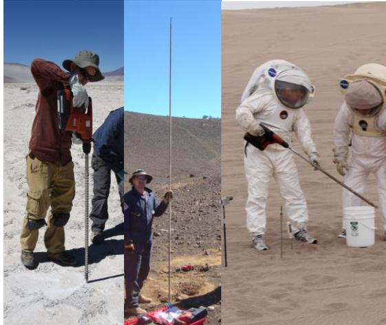
Figure 4. 1-5 m class drill deployed in various locations in planetary analog sites.
