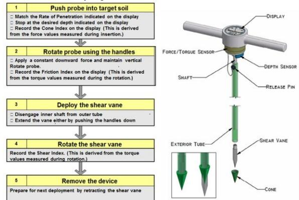
Figure 6. Stinger allows measuring of bearing capacity and shear strength independently.
