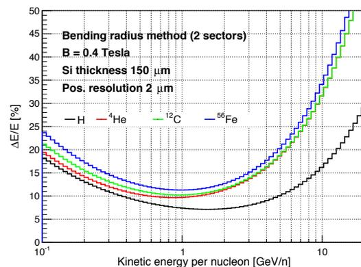
Figure 1. Energy resolution as a function of energy per nucleon for proton, Helium, Carbon and Iron nuclei from 100 MeV/n to 20 GeV/n, with the baseline Mini.PAN design.
