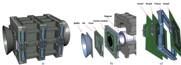
Figure 2. a) Engineering drawing of Mini.PAN. b) Exploded view showing the baffle, the TOF module coupled to the Pixel module, the tracker module and part of a magnet sector. c) Exploded view of a tracker module.
