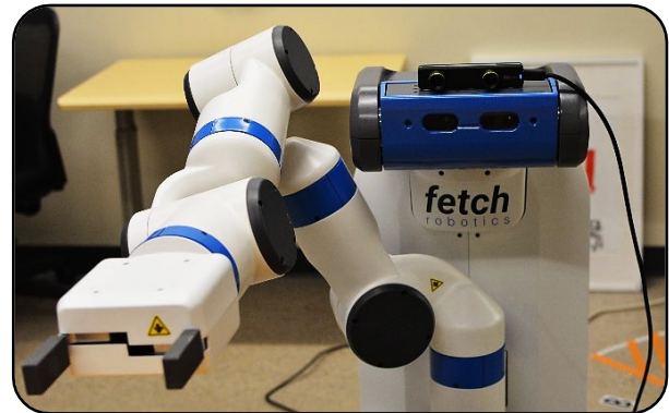
Figure 1: A Fetch Mobile Manipulator robot with a 7-DOF arm utilized for simulating long-distance teleoperation assembly tasks.
