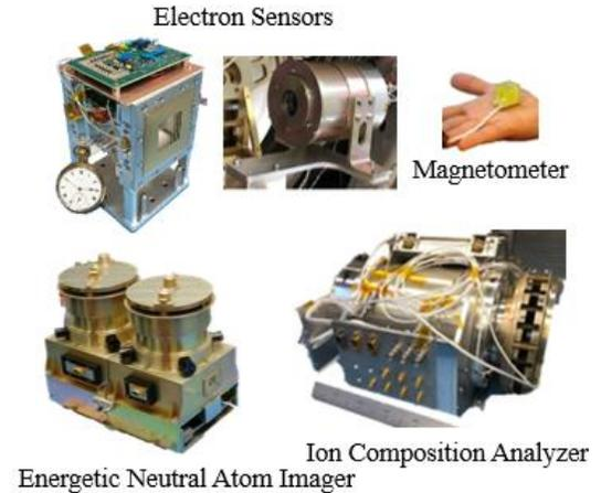
Figure 1. A plasma suite intended for deployment on the lunar surface.
