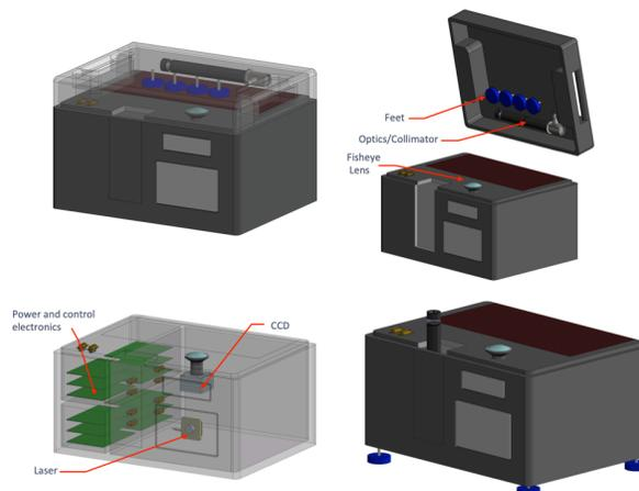
Figure 2. Isometric views of the sensor.
