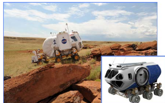
Figure 1. A proto-type small pressurized rover that has been tested in 3-, 14-, and 28-day long simulations of lunar missions with (inset) a concept flight vehicle.
