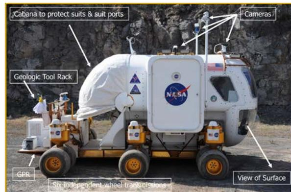
**Figure 1.** A ground penetrating radar (GPR) was installed beneath the aft deck of the Lunar Electric Rover, a terrestrial prototype of a Space Exploration Vehicle. The instrument was a technology demonstration component of a 14-day-long lunar mission simulation at Black Point, San Francisco Volcanic Field, northern Arizona.
