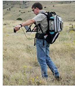
Figure 1: Symbolic picture of a surface reflectance measurement done with portable instrumentation (from SDMST.edu)
