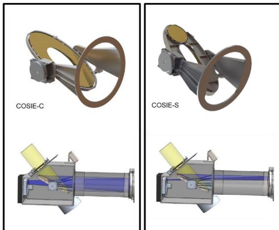
**Figure 5.** The COSIE instrument design combines a sensitive wide-field EUV imager and a slitless full-disk imaging spectrometer in a compact design.
