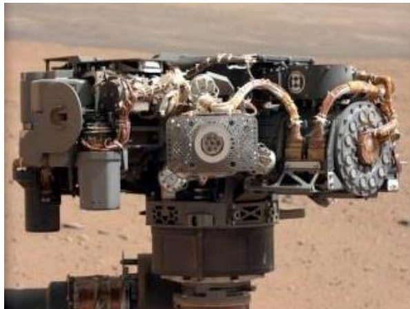
Fig. 1: APXS sensor head on the robotic arm of the Mars Science Laboratory (MSL) Curiosity Rover. Image Credit: NASA.
