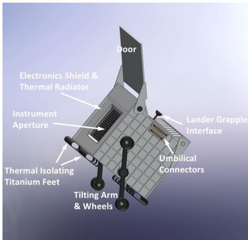
Figure 2. A CAD model of the EDA housing system.
