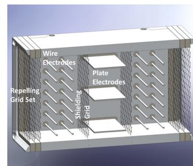
Figure 1. Top: Schematic of the EDA sensor; Bottom: Cut-view of a CAD model.
