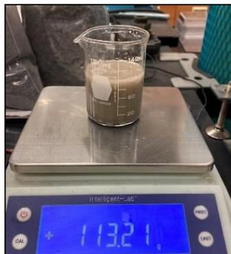
**Figure 1.** Flask with LMS-1 and Deionized Water
