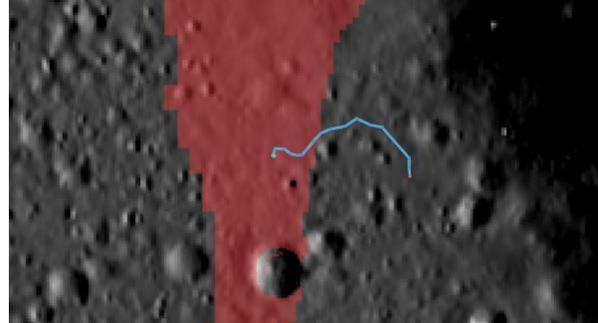
**Figure 2.** [Notional 3.6 km traverse](#) from landing site (Fig. 1) to a region inside the permanently shaded region on the floor of Amundsen with slopes <6°. Developed in the Lunar QuickMap tool.
