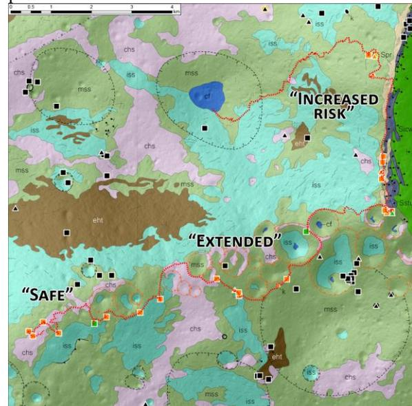
**Figure 1:** Excerpt of our geomorphic map (1:10,000) of Artemis III Areas of Interest 001 and 004 (Shackleton’s crater rim is on the right edge of the image). Dashed, red line is the three sequential traverses discussed in the text. Squares and triangles are blocks and blocky craters, respectively (orange: visited; green: approached; black: not visited or approached).
