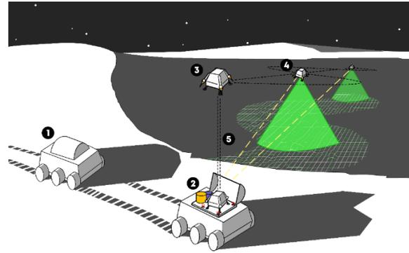
Figure 1: Illustration of the Lunar Reconnaissance Drone concept of operations: 1) standby mode, 2) flight preparation and deployment, 3) take-off and vertical ascent, 4) horizontal flight and mapping of the lunar surface, 5) vertical ascent and landing for data transmission, refueling, and standby. [2]
