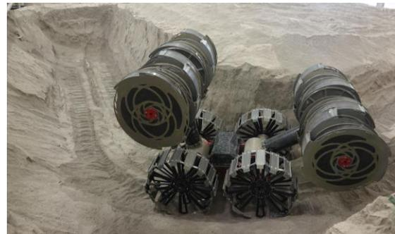
Figure 1. RASSOR excavating a slot trench in BP-1
