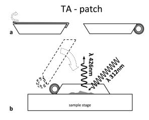
Figure 1: description of the TA patch proposed for TA assay a) removal of the seal from the TA patch before contacting it with the sample; 2) the TA patch is contacted with the sample and the TA-OH produced can be excited and the fluorescence detected thanks to the transparent container.
