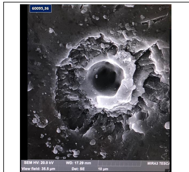
Figure 6: SEM image of a \sim 8 \mu\text{m} diameter micro-crater on sample 60095,36 with a spallation zone outside of the inner cavity and small sub-micron particles (dust) affixed to the glassy surface, likely related to the cratering event. With SEM, LCM, and xCT, the story of the finest scale lunar dust (nano-moon) can be measured and evaluated in the context of Artemis for both science and applied engineering purposes [7]. SEM image courtesy R. Kent (GSFC NDE).
