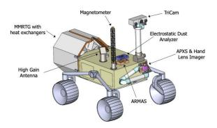
Here, we can distinguish the different main systems that compose a spatial rover. We can see: all terrain wheel, to explore the rocky surface of Mars, different instruments like a magnetometer, an electrostatic dust analyzer, to and analyze samples that the rovers will collect by using its digging and drilling tools.
