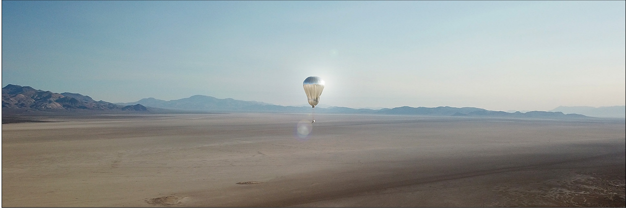
Figure 2. In July 2022, JPL and the Near Space Corporation successfully flight tested a one-third-scale, variable-altitude aerobot prototype. The aerobot ascended more than 1 km above the Black Rock Desert, where pressure and temperature are comparable to the conditions about 55 km above the Venus surface. Credit: Near Space Corporation.
