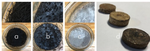
Figure 3. Bio-composites grown by redhouse. a) Dried Nostoc flagelliforme (diazotrophic cyanobacterium) in a sterilized glass jar. b) hydrated N. flagelliforme inoculated with A. oryzae liquid culture. c) fully
