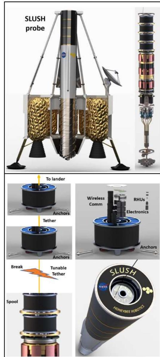
**Figure 1. Conceptual design of SLUSH. Top Right: SLUSH probe inside the lander. Top Left: SLUSH concept with internals visible. Bottom: Spool bay pucks house the tether. The pucks are left in the ice as the probe descends, remaining connected by the tether to provide communication with the surface. If the tether breaks, communication continues through the Tunable Tether approach.**
