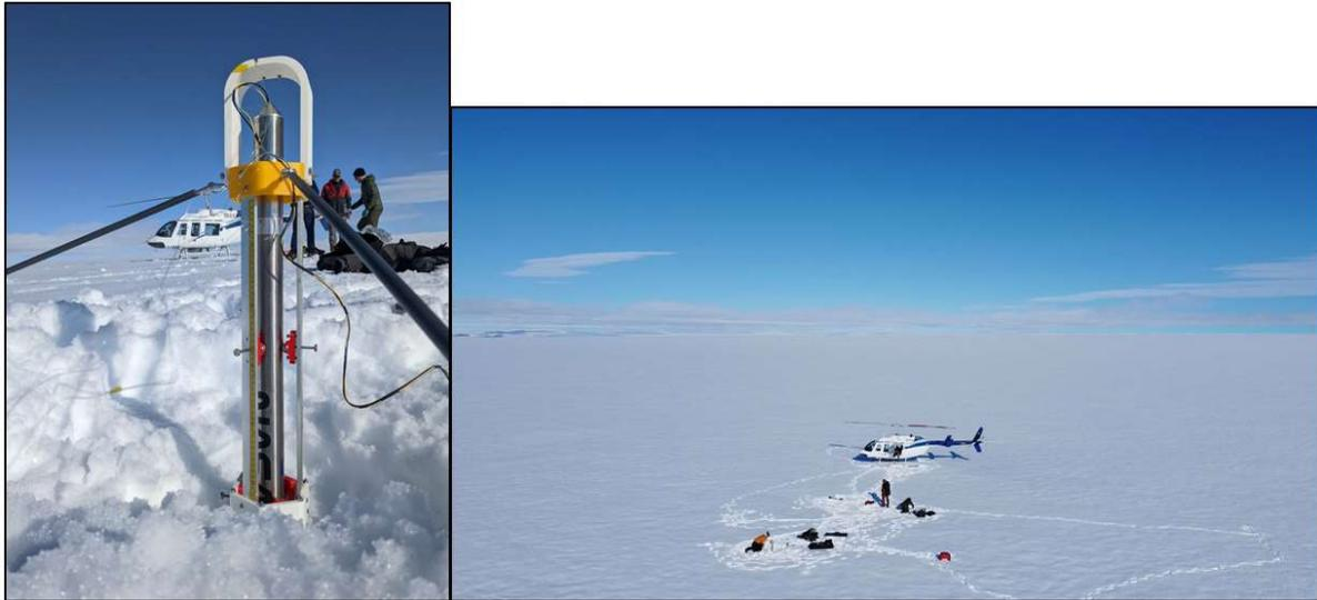
**Figure 2. Left: Honeybee Robotics' Salmon Probe set up on top of the Devon Island glacier before deployment into the ice. Right: Drone shot of the team on top of the glacier during testing.**
