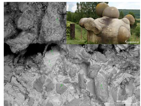
Fig.7. “Trovants” from Romania the sandstones of Costesti village. There are a type of sandstone concretion, up to 4.5 meters in diameter. The quartz grains cementation is primarily by calcium minerals. Microscope Sigma VP Zeiss. Top square- Romanian gigantic concretions „Trovants”. Image credit: https://www.geologyin.com/2018/04/the-mysterious-living-stones-of-romania.html
