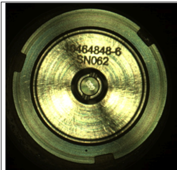
Figure 5. Cachecam image of a sealed sample tube containing the Malay sample (Sol 337).
