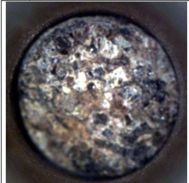
Figure 4. Cachecam image of the Malay core tip (Sol 337). The sample core is ~ 13 mm in diameter.
