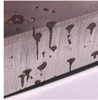
Figure 1: Photograph of Smithsonian slice of Dronino showing various sulfide features (USNM 7203). Thickness of slice = 2 cm.
