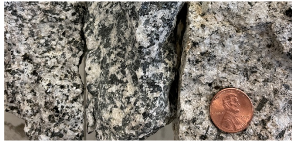
Figure 1: Granodiorite (left), tonalite (middle), and granite (right) from intrusive sample suite. Shown in Figure 2 left panel as green, black, and green spectra respectively. These range from \sim 60\text{-}72\ \text{SiO}_2\ \text{wt}\% and \sim 15\text{-}45\ \text{plag}\ \text{wt}\% .
