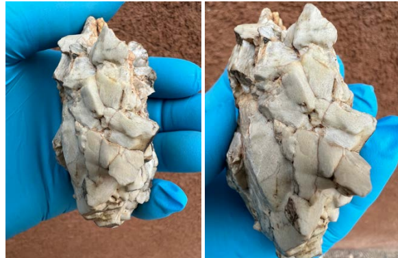
Fig. 3. Photographs of the 216 gram deposit sample of Sebkhah el Melah 001 showing a cluster of interlocking single crystals enstatite.
