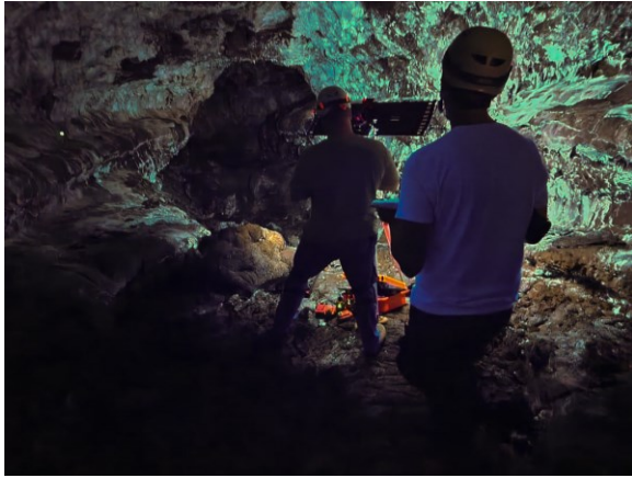
Figure 2. Field image showing the UVIF system in operation. The right lava tube wall is directly illuminated by UV showing bright green and blue fluorescence. Photo credit: NASA Expeditions.
