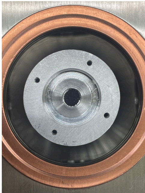
Figure 1. Ryugu powder samples in sample holder. The sample cup (center) is 5mm in diameter.
