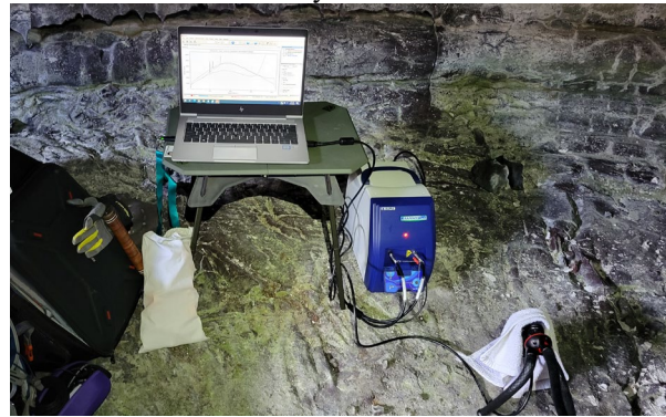
Figure 2 – The iRaman plus instrument setup inside the lava tube with the laser in the lower right connected to the detector in the blue and gray case.
