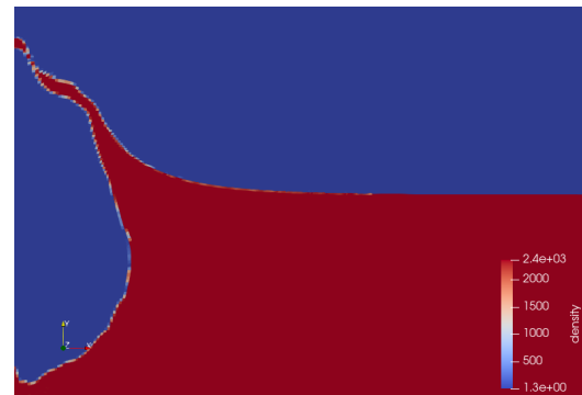
Figure 2: Screen capture of the strengthless simulation at 3.6 s, colored by density. At this time, the surface of the alluvium breaks.
