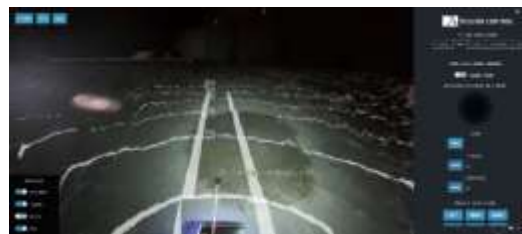
Figure 2: A screenshot of the Mission Control Software operations interface used in the challenge, highlighting how distance estimation tools were used by the team for evaluating decisions for navigation and instrument targeting.
