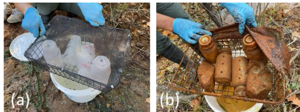
Fig. 1: Samples before (a) and after (b) exposure to field ARD. Perforated Nalgene 500 mL bottles containing the dialysis membranes with nontronite or silicon oxide were secured in custom-made metal cages and submerged into ARD at the Tab-Simco ARD site in southern Illinois.
