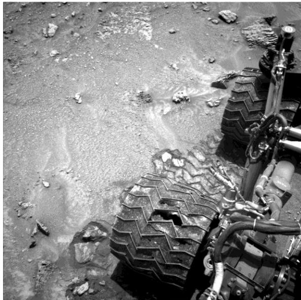
Figure 1 – The wheel condition of Mars Curiosity on sol 3672 (5 December 2022). Credits: NASA/JPL-Caltec [1]
