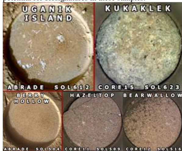
Fig. 1: Images of rocks of Yori Pass (top) and Hogwallow Flats (bottom). Abrasion patches Uganik Island and Berry Hollow on left. Cores Kukaklek, Hazeltop, and Bearwallow in center and right.
