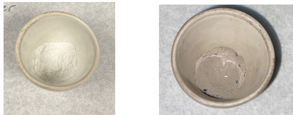
Figure 3: Wollastonite sample before (left) and after (right) reacting in the Venus simulation chamber for 10 days. The gleaming particles in the right sample are pieces of the graphoil gasket in the chamber that flaked into the ceramic bowl.
