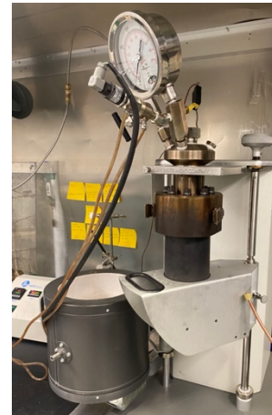
Figure 1: Venus Simulation Chamber (Cassiopeia chamber) is located at the center in a holder. The heating sleeve is towards the bottom left, and the pressure gauges are located at the top of the system.
