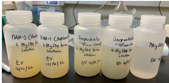
Figure 1: Batch dissolution experiment set-up for nontronite and serpentinite. Note that there is one duplicate for each mineral sample and a blank.
