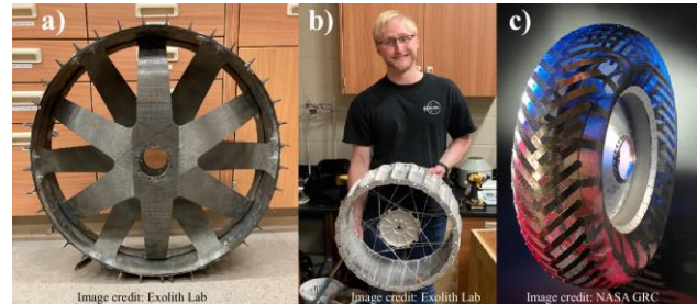
Figure 2. Three lunar rover vehicle wheels to be used for GATOR trafficability experiments. (a) Astrobotic Technology Polaris rover prototype, (b) NASA Glenn Research Center (GRC) VIPER-like (Resource Prospector) prototype (Jared Long-Fox for scale), (c) and the coolest of all three, GRC Apollo Lunar Roving Vehicle (LRV) replica tire.
