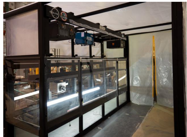
Figure 1. The RIDER test rig is housed at UCF CLASS Exolith Lab and is a custom-built gravity offloading trafficability testing rig (3.8 m x 1 m x 1.7 m tall) designed to test wheel-regolith interactions. RIDER will be operational in early 2023.
