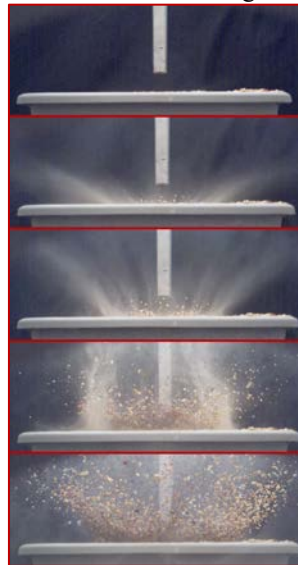
Figure 1. Snapshots of a gas cratering experiment using the APL PIL configured to perform gas-only experiments on a coarse particle target that has a small fraction of dust. Note the early onset of dust ejected at shallow angles. The dust ejection angle steadily steepens with time. The coarse particles are mobilized more slowly than dust and have a fixed ejection angle.
