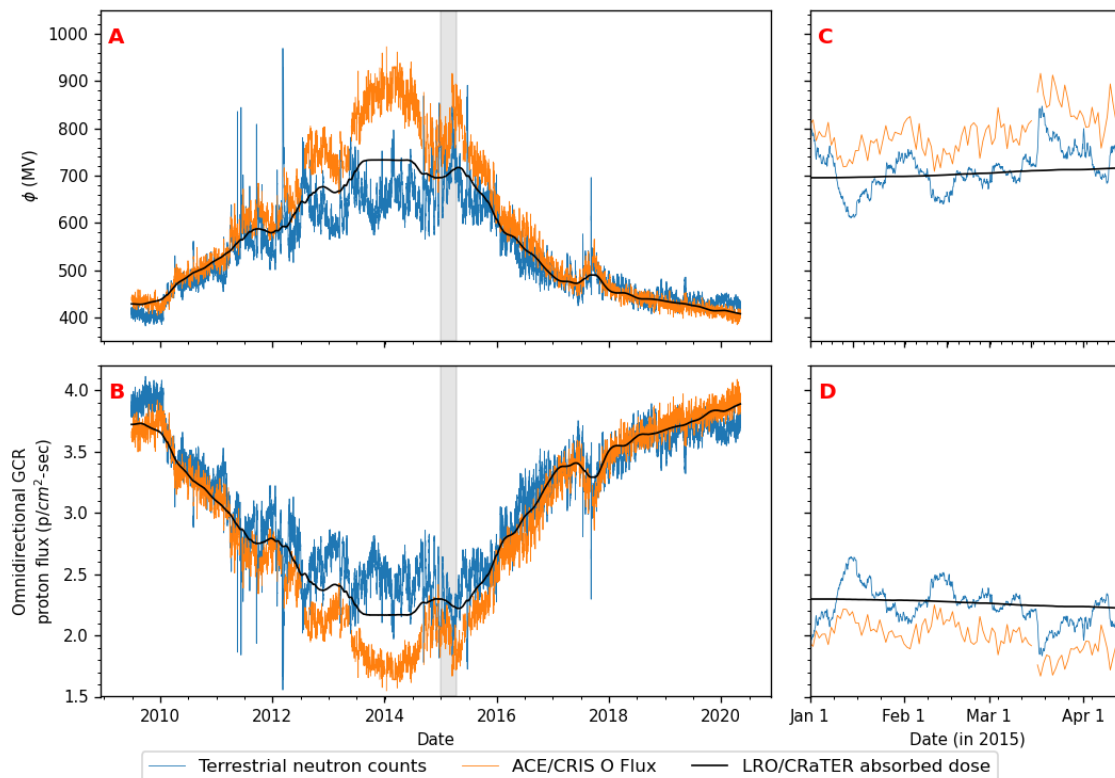
Figure 2. (A) Solar modulation potential as estimated from terrestrial neutron count rates (blue), GCR oxygen flux from ACE/CRIS (orange), and absorbed dose from the LRO/CRaTER instrument (black). Data are shown for most of the last solar cycle, starting with the launch of LRO in June 2009. (B) Omnidirectional GCR proton flux for the \phi in (A), computed using the differential GCR flux spectrum formulation provided in [6] and integrated over 10 to 10^6 MeV. (C,D) Same as (A) and (B), but for a window during the peak of the last solar cycle (January to April 2015, gray vertical shaded areas in A,B) to show variability in solar modulation and the corresponding estimated proton flux for a VIPER-like mission duration (~100 days) [1]. VIPER is expected to be operating at the lunar south pole during the peak of the next solar cycle (~2024–2025).
