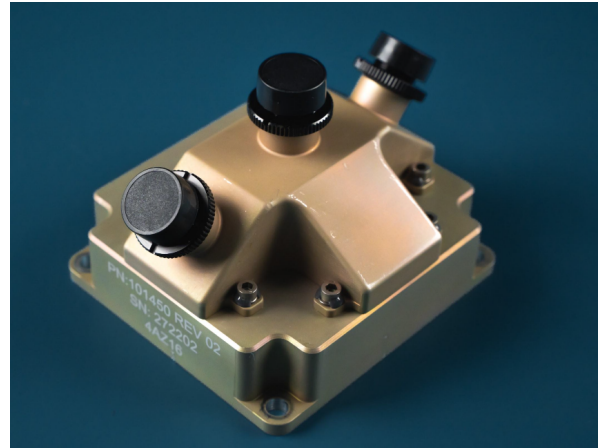
Fig. 1. VCA engineering model, showing a single cluster of three cameras. VCA is being built by Redwire Space and consists of three clusters positioned around the lander for 360° coverage. The camera housing is 3.1 × 3.26 inches at its base.
