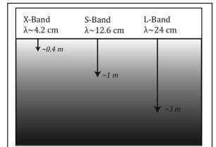
Figure 2: Comparison of radar wavelength and approximate penetration depth at the lunar south pole from LRO's Mini-RF instrument (X-band and S-band) and Chandryaan 2's DFSAR instrument (L-band).
