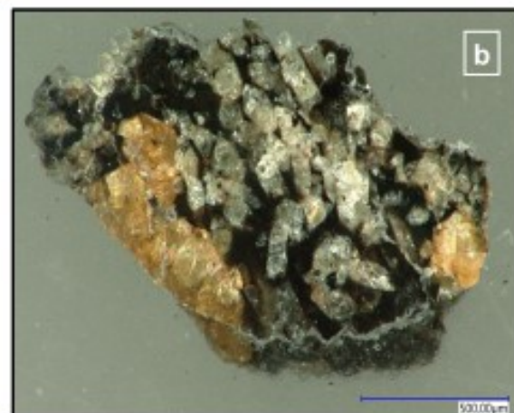
Figure 3(a): Erg Chech 002 [5], ungrouped achondrite: terrestrial quartz particles in small pockets. (b) Yamato 980459 olivine phyric shergottite [5]: lower shock of 20-25 GPa, orange olivines.
