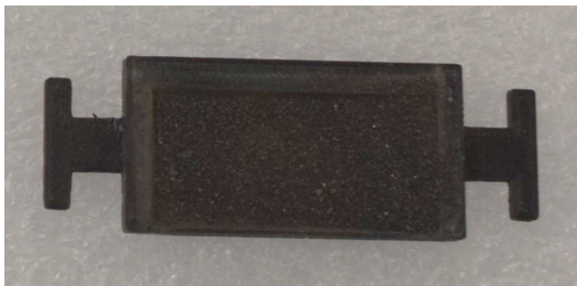
Figure 2. Example of a regolith sample (JSC-1A lunar simulant) collected and prepared for in-situ analysis.
