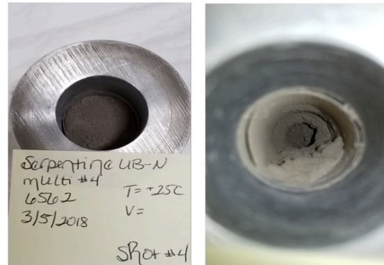
Figure 1. (Taken from [11]). Images of the serpentine sample after the fourth impact (left), along with the crater produced by the impact (right). The crater is 60 - 70 mm deep. The shot velocities for this experiment ranged between 2.41 to 2.44 km/s, a total of 6 shots were made into this sample.
