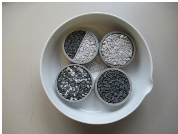
Figure 1. The two end-members and the two 50%+50% mixtures (spatial and intimate, both in volume) in the ceramic sample holders used for emissivity measurements.
