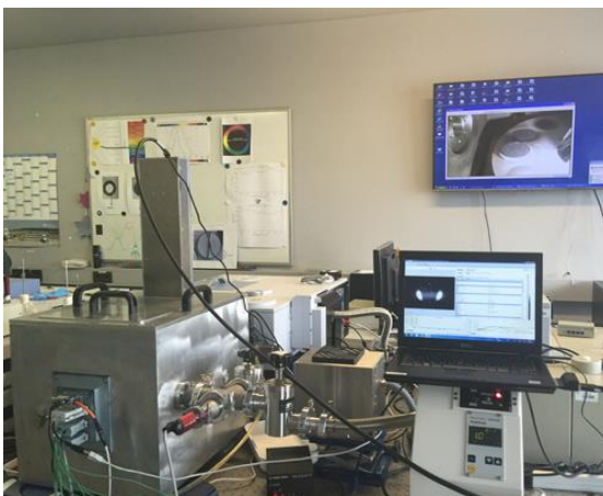
Figure 2. The VEM/VenSpec-M prototype on top of the Venus emissivity chamber at PSL during measurements to verify instrument performance.
