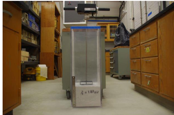
Figure 1. Rimik CP40II CPT insertion into LHS-1B “Simplified” lunar highlands simulant column packed within a clear, acrylic test bin at \rho_B = 1.83 \text{ g/cm}^3 (12” ruler for scale).
