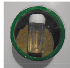
Figure 3. The middle compartment. It contains sand (from the Danube). The cover of the compartment can be removed with a twisting movement.
